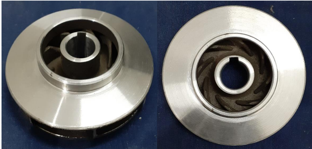
Fig. 3.0.1. Impeller manufacturing via sand casting method
