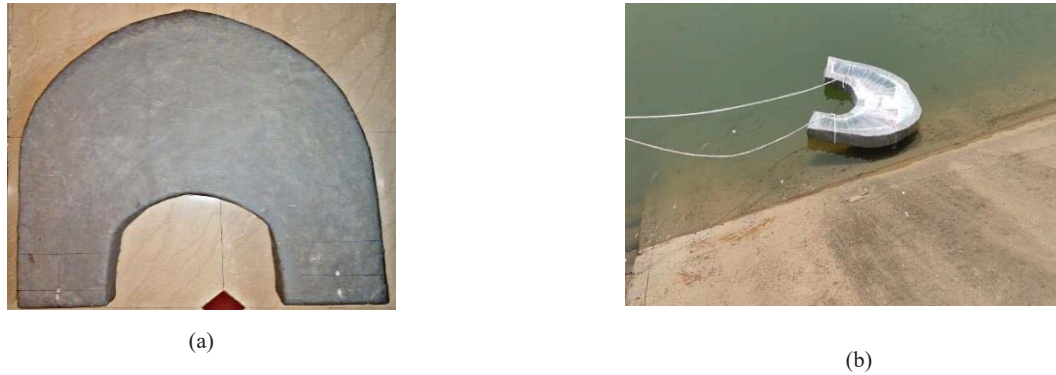
Fig.12. (a) final product (b) hull is floating on water
