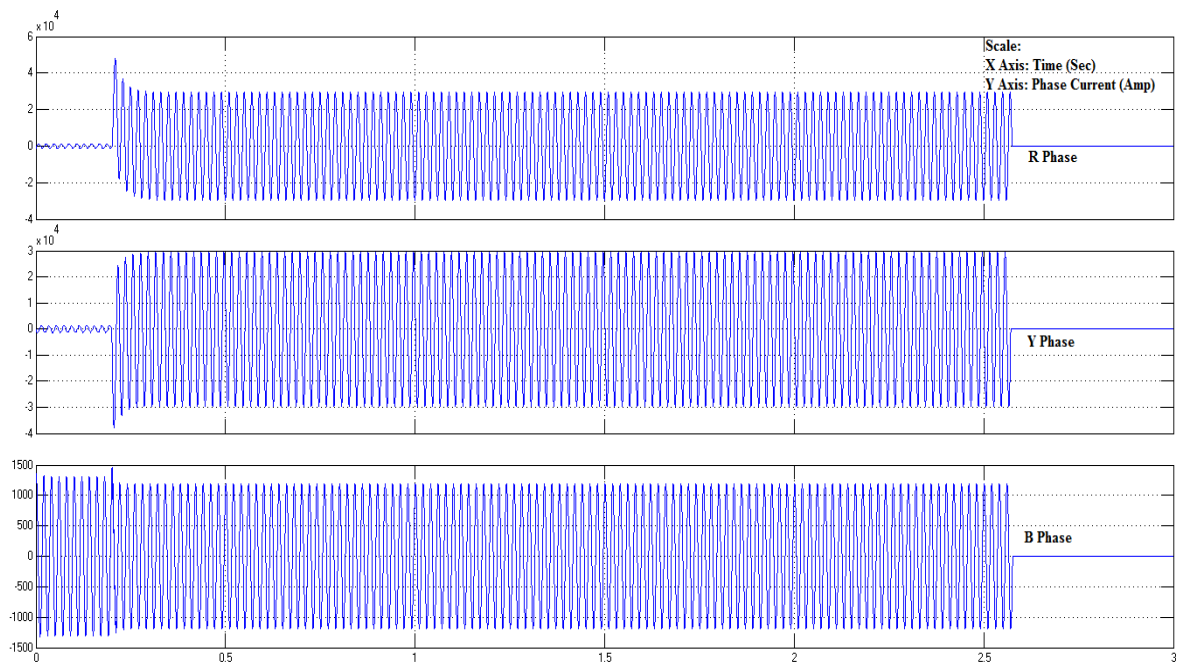
(a) Fig 6 Standard Inverse Response (a) Phase Current Vs Tripping Time (b) Tripping Signal (approx. at 1.05 Sec)
