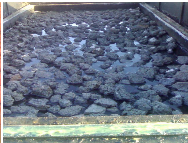
Fig. 12 Photograph of the still with 1½ in. cement concrete used in the basin [8]
