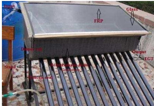
Fig. 17 Schematic diagram of solar still coupled with evacuated glass tubes [10]
