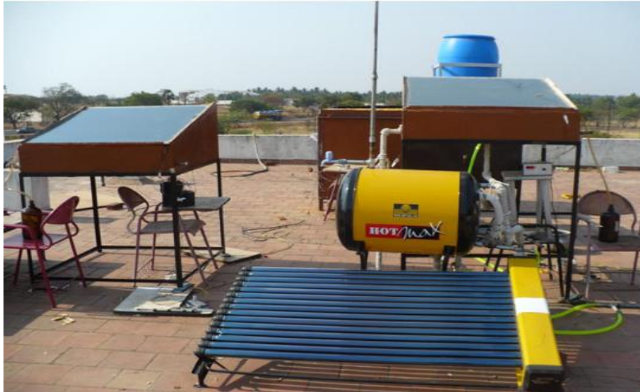
Fig. 10. Photographic view of solar still coupled with solar water heater [10]
