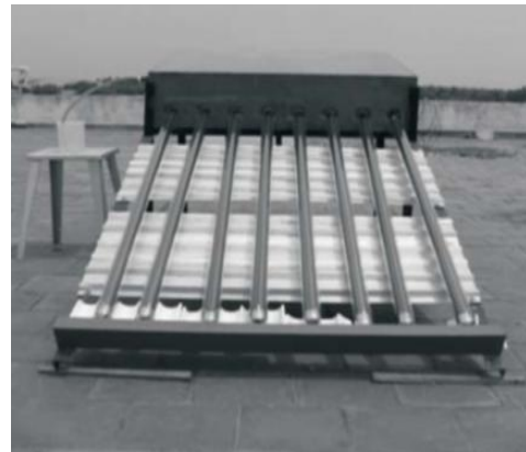
Fig.3. Pictorial view of solar still augmented with evacuated glass tubes [4]
