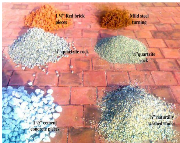
Fig. 11 Photograph of sensible energy storage materials pieces in the basin [8]
