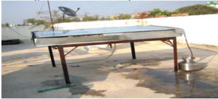
Fig. 3 Photographic view of black granite single basin solar still [5]
