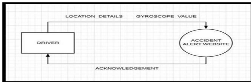
Fig. 1. Level 0 DFD (Data Flow Diagram)
