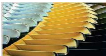
Fig.8. Coated turbine blades.
