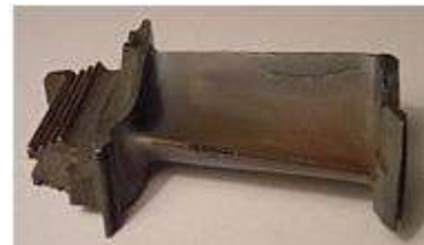
Fig.3. Nickel Super alloy jet engine turbine blade.
