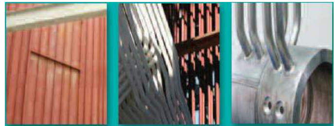
Fig.6. Membrane wall, Tubes and SH outlet header.
