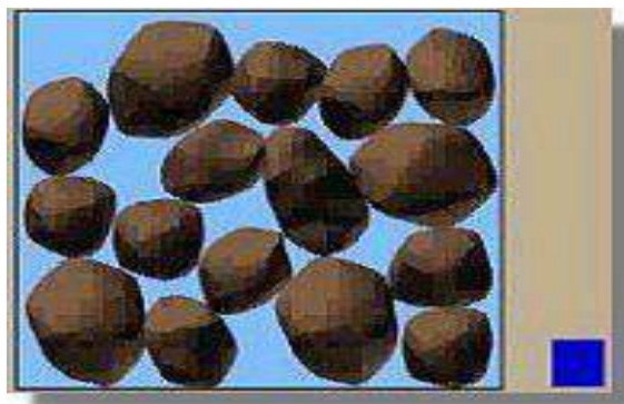
Fig.1. (a) Soil grains in a soil deposit. The height of the blue column to the right represents the level of pore water pressure (Reference: www.ce.washington.edu/~liquefaction )
