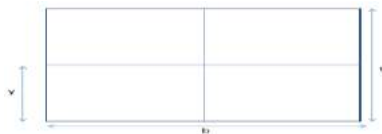
Figure 4.1 rectangular cross section of leaf spring
