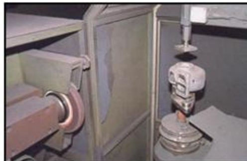
Fig.5. Inside the fettling machine showing a casting mounted in a fixture and the grinding wheel.
