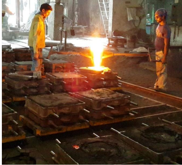
Fig. 2. Manual molten metal pouring process in traditional foundry.
