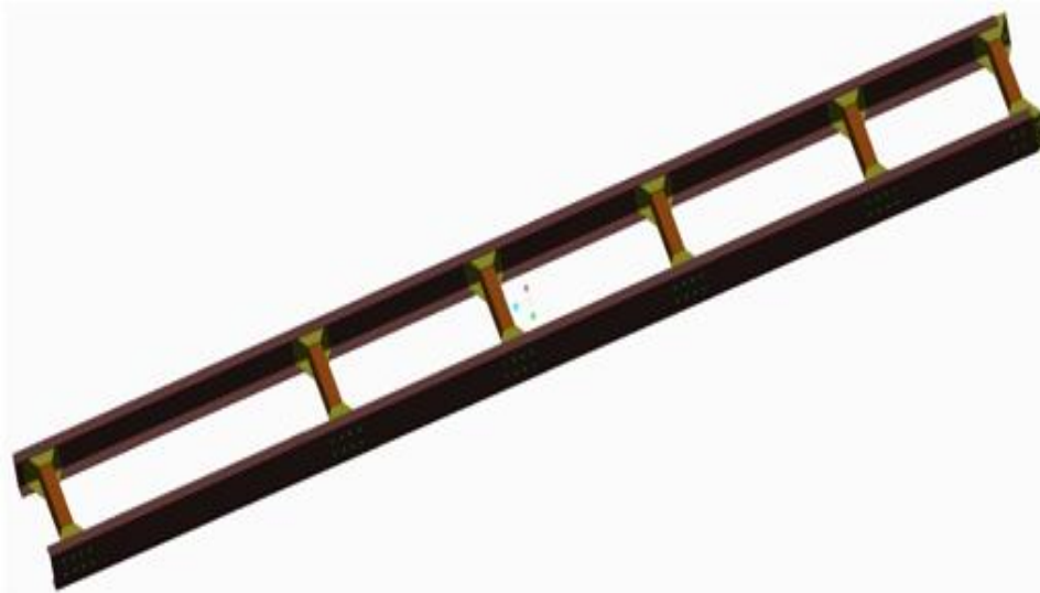
Fig. 2: CAD model of chassis in PTC Creo 3.0
