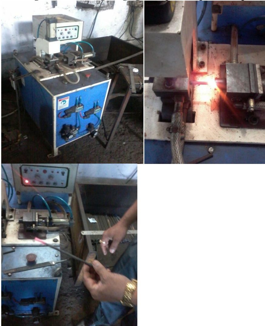
Figure No-08:Tang Forging Set Up with Special Purpose Resistance Heating Furnace
