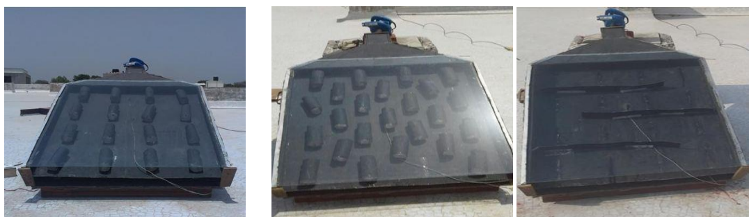
Fig. 1 Experimental Setup of SAH (a) Type - I (b) Type - II (c) Type - III.
