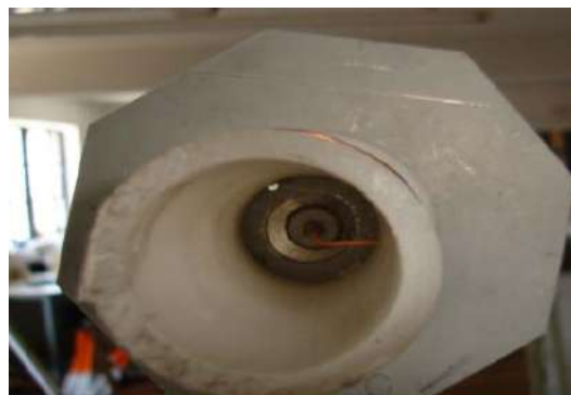
Figure 6. Helical antenna with ground plane.
