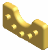
Figure 6 Circular pattern of cylinder on part
