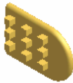
Figure 5 Rectangle pattern of rectangle block on part
