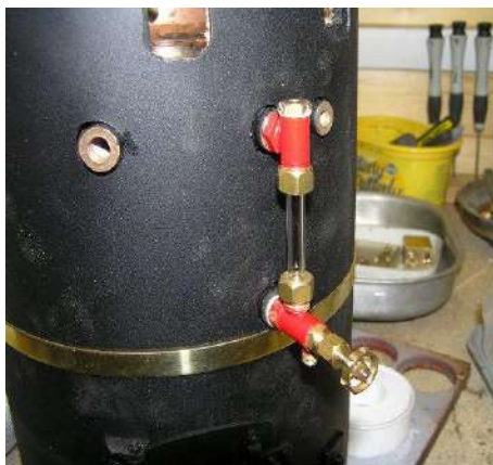
Figure 3 Water gauge fixed to boiler
