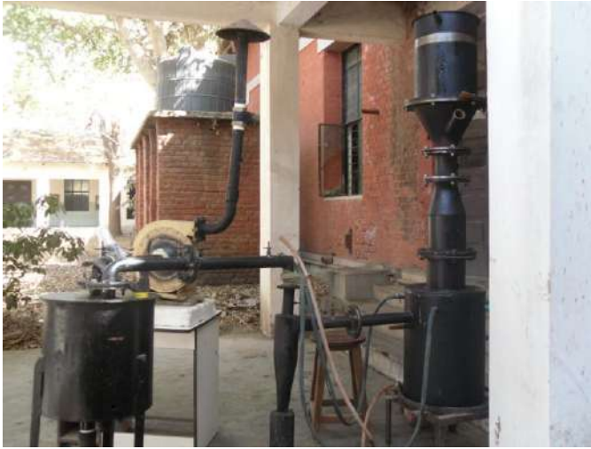
Fig.3 Venturi Type Gasifier at L D Collage O Engineering with cyclone separator, wood filter & blower ready for testing.
