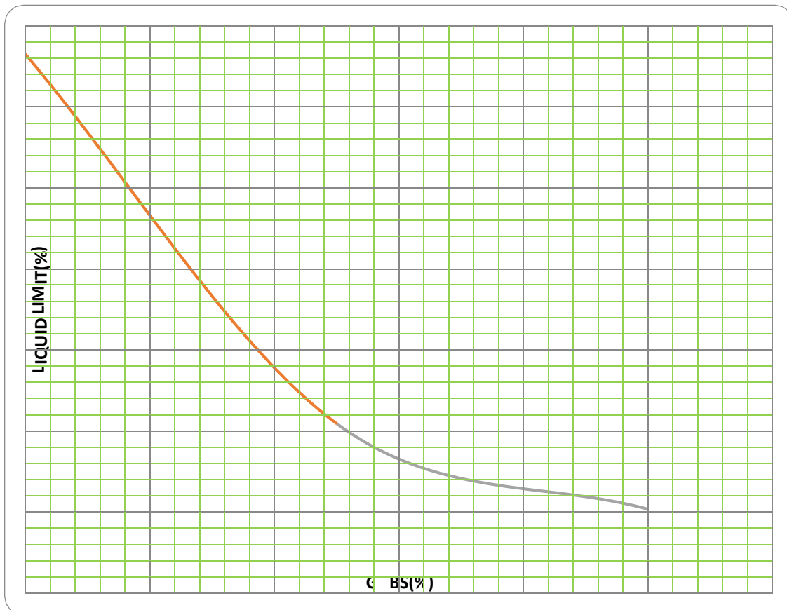
Fig. 3. Graph.of GGBS(%) vs. Liquid limit (%)
