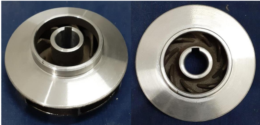
Fig. 3.0.1. Impeller manufacturing via sand casting method
